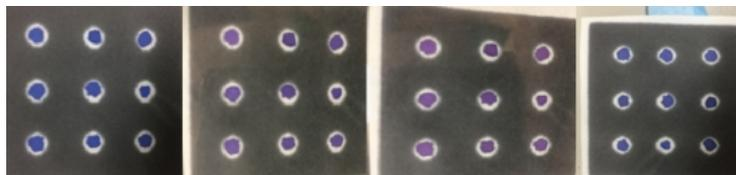
Figure 2.11: While this protein initially appeared blue (left), it begins to turn purple at 55 °C (center left) and this purple color becomes more pronounced as temperature is increased (center right). Interestingly, when allowed to cool back to room temperature, the blue color returned (right).
